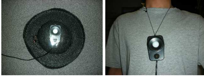
Figure 3.4: Left: Light Sensor on a Hat. Right: Light Sensor as a Pendant
