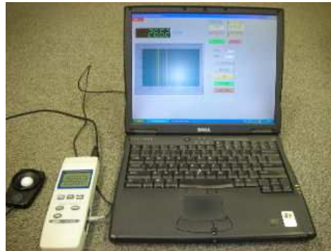
Figure 3.5: Apparatus Used for Data Collection for Light-based Localization
