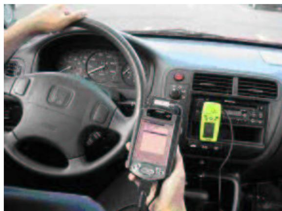
**Figure 3. EZCab driver station consisting of an HP iPAQ equipped with Orinoco 802.11 wireless card and Geko 201 GPS receiver**
