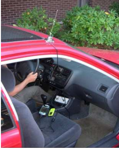
Figure 1. TrafficView Prototype Installed in a Car
