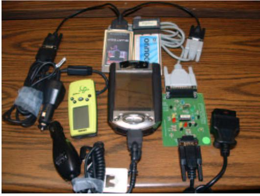
Figure 3: TrafficView prototype hardware components
